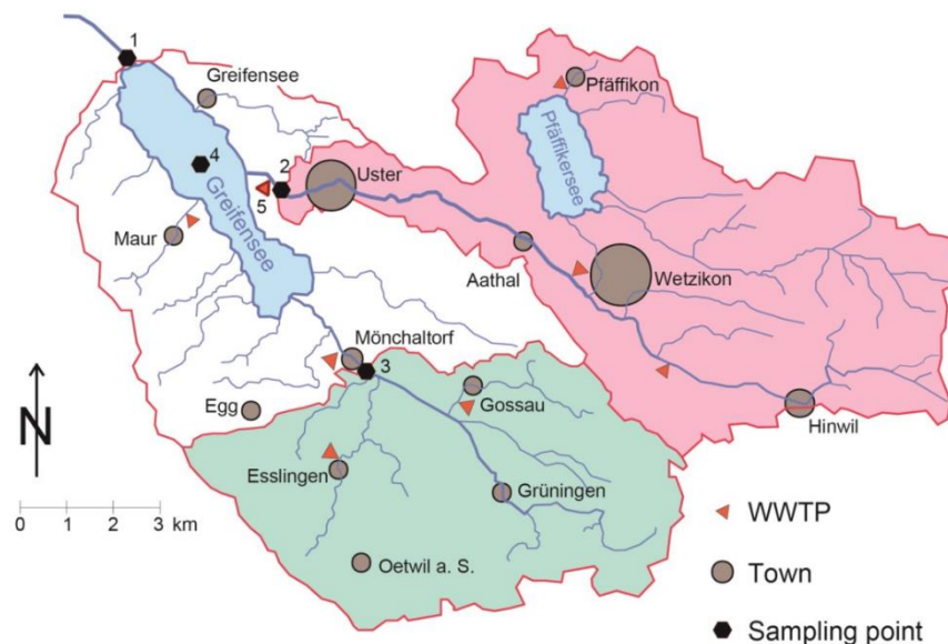
Figure 8.5-82: Map of the catchment area of Lake Greifensee with sampling points. Weekly flow-proportional composite samples were obtained from the automatic sampling stations at the tributaries to the lake, Aa Uster (2) and Aa Mönchaltorf (3) as well as the outflow from the River Glatt (1). Monthly grab samples from several depths were taken at the deepest point of the lake (4). Daily flow-proportional composite samples of treated wastewater were obtained from WWTP Uster (5). The sub-catchments discharging at the sampling points 2 & 3 are marked in red and green, respectively.
